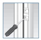
Adjusting the SCREEN **ROLLERS.** Tighten to lift and loosen to lower.
